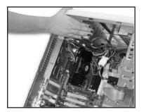
**Step 4**With the power cable disconnected from your computer, touch the metal part of the case to ground yourself. This will discharge any static electricity from your body which can damage your computer.
